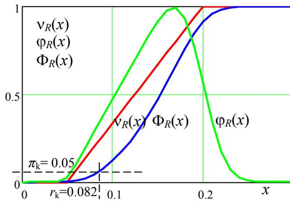
**Figure 2.** The membership function  $v_R(x)$ , the damage function  $\Phi_R(x)$  and the damage density function  $\varphi_R(x)$  for the transition region from  $r_1 = 0.05 \text{ mm}$  to  $r_2 = 0.2 \text{ mm}$  and  $V_R = 0.10$
