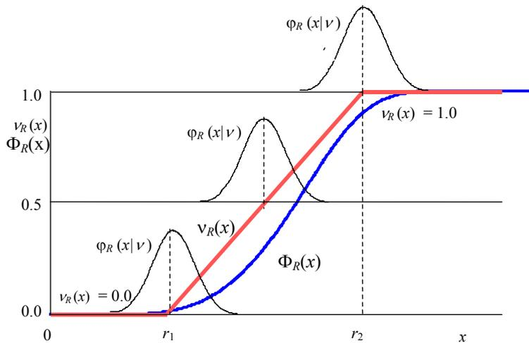
**Figure 1.** The fuzzy probabilistic model of the performance requirement  $R$
