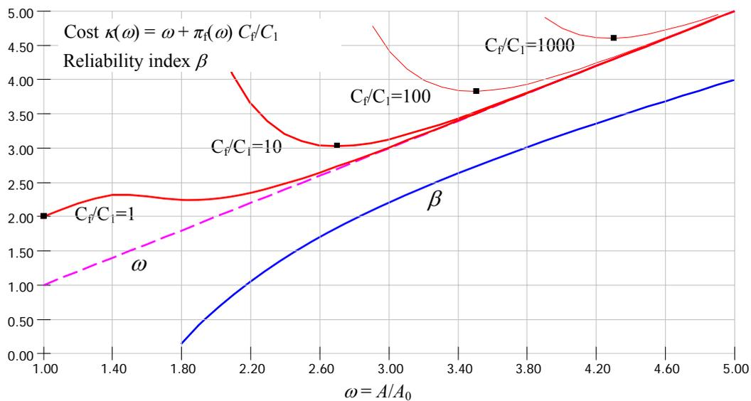
**Figure 4.** Variation of the total normalized cost  $\kappa(\omega)$  and reliability index  $\beta$  with the reinforcement ratio  $\omega$  for the reinforcement diameter  $\phi = 16 \text{ mm}$
